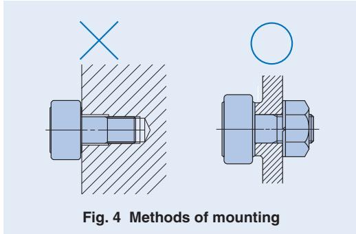
Fig. 4 Methods of mounting
