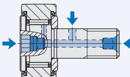
Grease nipple is incorporated in the stud head.
