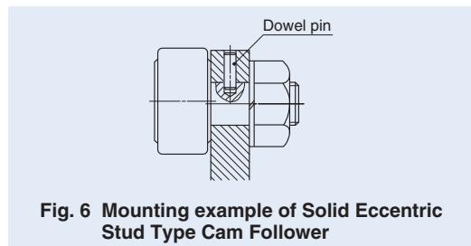
Fig. 6 Mounting example of Solid Eccentric Stud Type Cam Follower
