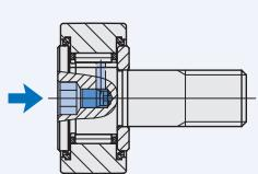
Re-greasing fitting is incorporated in the stud head.
