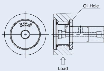
**Fig. 2 Oil hole position and loading direction**
