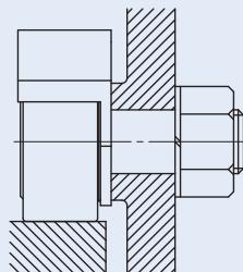
**Fig. 9 Mounting of C-Lube Unit**
