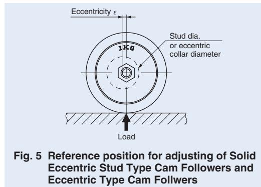
Fig. 5 Reference position for adjusting of Solid Eccentric Stud Type Cam Followers and Eccentric Type Cam Followers
