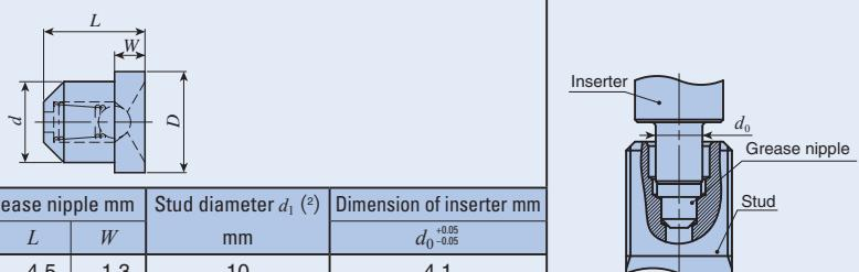
Notes<sup>(1)</sup> Applicable to Cam Followers other than Inch series Cam Followers.<sup>(2)</sup> For Eccentric Type Cam Followers, thread diameter G as shown in the dimension table is applicable.<sup>(3)</sup> Only applicable to Standard Type Cam Follower CFKR, and Eccentric Type Cam Follower CFKRE sizes 22 and 26.
