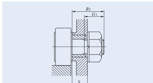
Fig. 7 Length of the mounting hole of Eccentric Type Cam Follower
